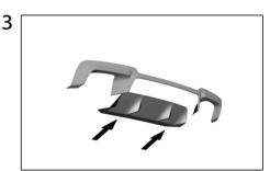
Replace the OEM diffuser with Sterckenn Diffuser.
