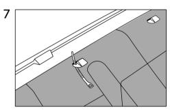
Use attached zip ties and run them thru the hole. This will lock and place the Sterckenn Diffuser tight with OEM diffuser.
