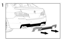
Remove three 8mm screws located toward the center part of OEM diffuser. Then start pulling down outside corners of the diffuser to releas it.
