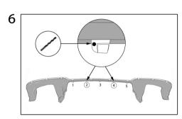
Use attached drill to make a hole in marked spot. (Remove Sterckenn Diffuser to avoid damaging the part)
