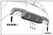
Align the Sterckenn Diffuser mounting holes and install all three 8mm screws that were removed before. Push the outside corners of OEM diffuser up to lock it's position.
