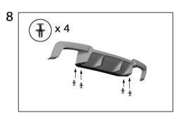
Position and lock Sterckenn Diffuser by using 4 black fixing plugs attached to this mounting kit. 9
