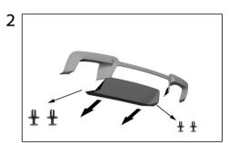
Remove 4 black fixing plugs located on the corners of the black OEM diffuser and detach diffusers from each other.
