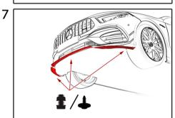
Align the Sterckenn splitter mounting holes. Install 11 bolts and 5 screws that are attached to this mounting kit.
