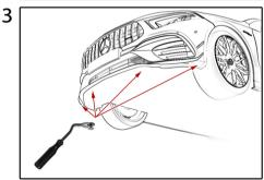
Remove 8 OEM plastic rivets for better access inside the bumper.
