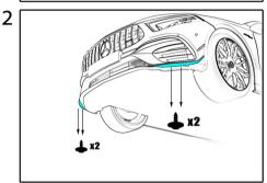
Remove OEM mounting screws from the bottom of side splitters.
