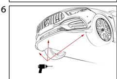
Drill holes marked before. Hole located in the center of this splitter (number 6) requiers smaller drill (bolt 4x12).
