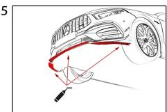
Mark 11 spots necessary to drill the holes later on. Check the attached printout.
